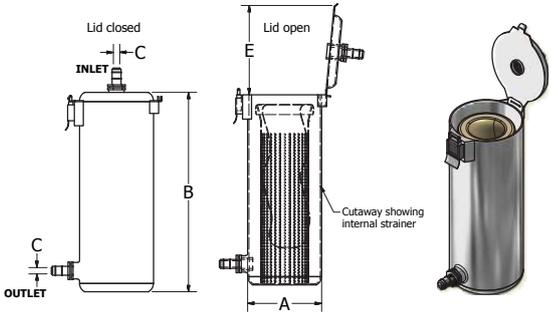
INLET/OUTLET connections available for 16mm and 20mm ID. Allow minimum clearance required for servicing as per table below (E).
